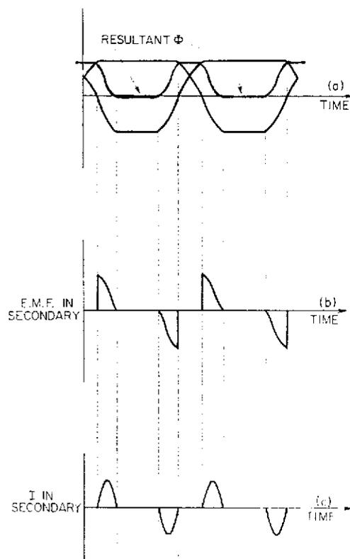
FIG. A.II.18. Resultant flux, e.m.f. and current in secondary
